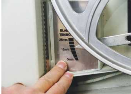
▲ Tensioning can be assessed with the indicator
